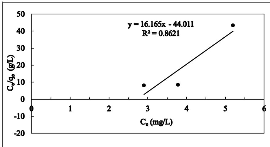
**Figure 1.** Langmuir isotherm plot for the adsorption of Pb(II) ions onto the mixture of sugarcane bagasse and banana peels.
