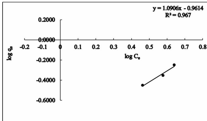
**Figure 2.** Freundlich isotherm plot for the adsorption of Pb(II) ions onto the mixture of sugarcane bagasse and banana peels.
