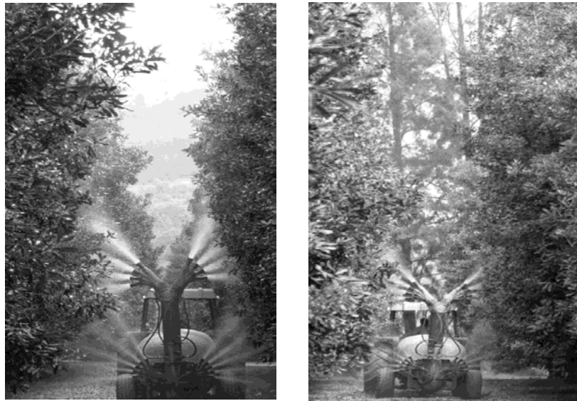
Fig. 1. Example of commercial orchard sprayers not able to reach the preferred habitat of phytophagous stink bugs in the tops of mature macadamia trees.
