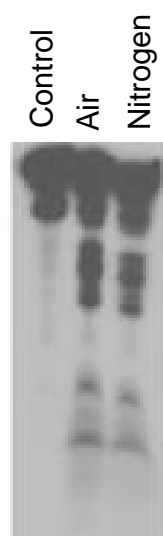
Figure 3. Comparison of DNA photodamage induced by RD-6G under air or nitrogen. The reaction mixture contained the ^{32}\text{P} -5'-end-labeled 211 bp DNA fragment, 10 \mu\text{M}/\text{bp} of calf thymus DNA, 50 \mu\text{M} RD-6G, and 2.5% (vol) ethanol in 100 \mu\text{L} of 10 mM sodium phosphate buffer (pH 7.8). The reaction mixtures were irradiated (365 nm, 6 \text{J}/\text{cm}^2 ). Then, the DNA fragments were treated with piperidine and analyzed by electrophoresis.
