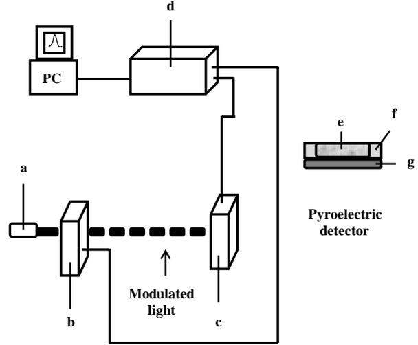
**Figure 2.** Experimental scheme for the inverse photopyroelectric technique. The elements correspond to: a) He-Ne laser, b) Acousto-optic modulator, c) Photopyroelectric detector (shown in detail in the right figure), d) Lock-in amplifier. Details of the detector: e) Dygline sample, f) sample container (O-ring), g) PVDF pyroelectric detector.
