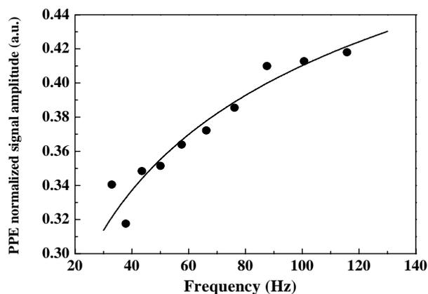
**Figure 4.** Photopyroelectric amplitude signal as a function of the incident light beam frequency. The solid line corresponds to the best fit of complex equation (3) with the normalized amplitude signal.
