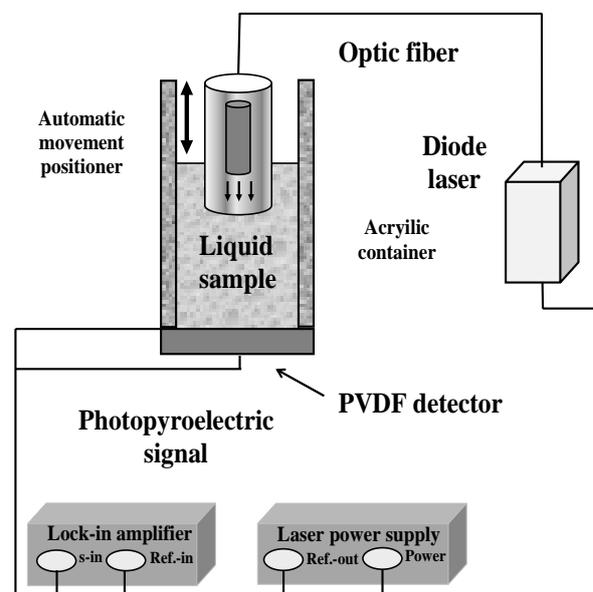
**Figure 1.** Experimental arrangement used for thermal diffusivity measurement of Diglyme.
