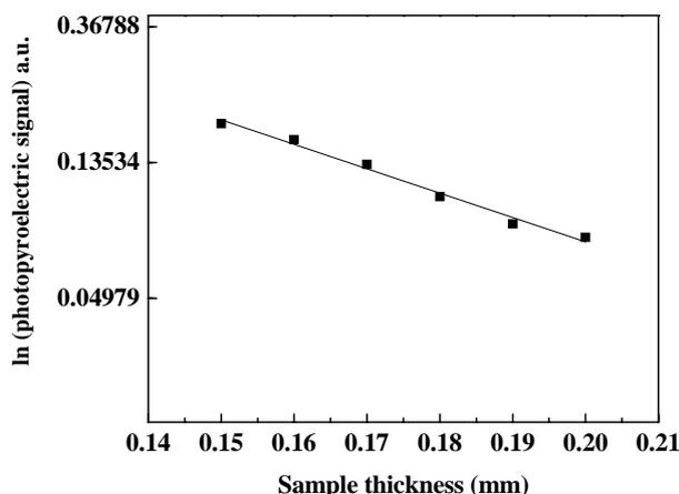
**Figure 3.** Ln (PPE signal) as a function of sample thickness. The symbols correspond to the experimental data and the solid line is the best fit of the equation (2) with the experimental data.
