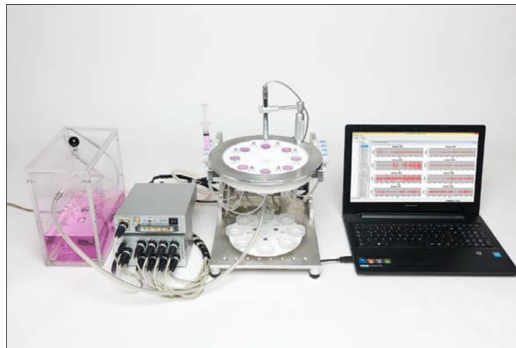
Fig. 1. The Microimpedance Sensor System (MSS): Photograph: A. Stertzik. From left to right: reservoir with water (stained in pink for photography only), pump and electronic unit, chamber array set-up with 8 individual flow-through chambers and USB-camera on the top, laptop with specific software for data recording and analysis.
