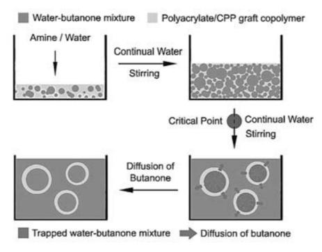
Figure 3. Schematic formation mechanism of hollow microspheres via the phase-inversion method. Reprinted with permission from Cao, Y. *et al.*, Langmuir, 26(9), 6115-6118. Copyright (2010) American Chemical Society.
