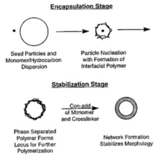
**Figure 4.** Schematic of two-stage voided latex particle process. Reprinted with permission from McDonald, C. J. *et al.*, Macromolecules, 33, 1593-1605. Copyright (2000) American Chemical Society.
