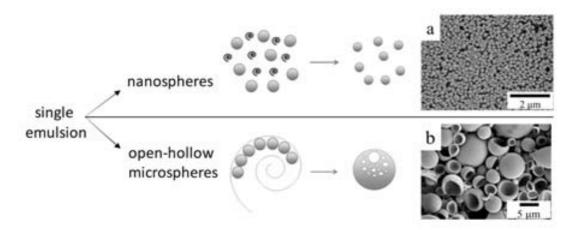
**Figure 2.** Transitional behavior of polymeric hollow microsphere formation in turbulent shear flow by emulsion diffusion method. Reprinted from Ji, S. *et al.*, Polymer, 53, 205-212, Copyright (2012) with permission from Elsevier.
