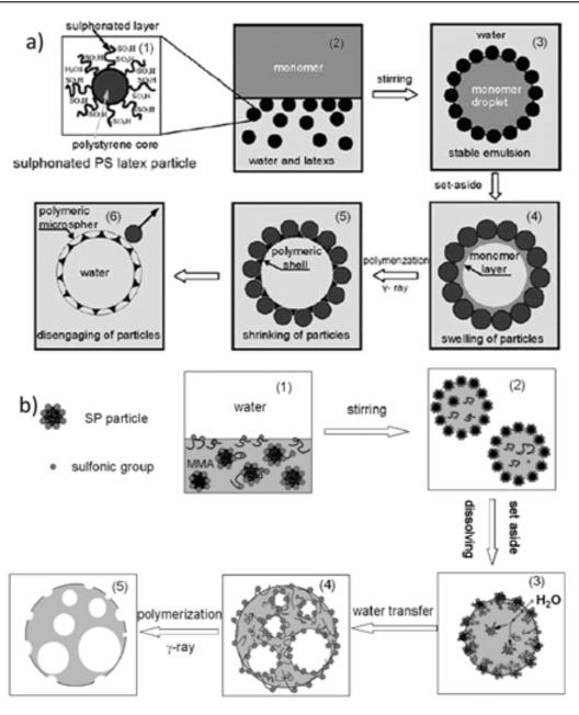
**Figure 7.** Schematic illustration of the formation of cage-like a) and multiple multihollow structure b) microspheres. Reprinted with permission from Yuan, Q. *et al.*, Langmuir, 25, 2729-2735. Copyright (2009) American Chemical Society.
