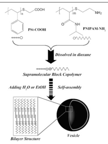
**Figure 5.** Illustration of vesicle formation from supramolecular block copolymers. Reprinted with permission from Qian, J. and Wu, F. P. Macromolecules, 41, 8921-8926. Copyright (2008) American Chemical Society.
