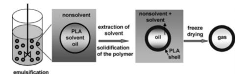
**Figure 1.** Schematic representation of the emulsion solvent-evaporation/ extraction preparation method of hollow PLA microcapsules. Reprinted from Sawalha, H. *et al.*, Chemical Engineering Journal, 169(1-3), 1-10, Copyright (2011) with permission from Elsevier.
