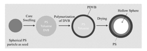
**Figure 8.** Formation mechanism of monodispersed hollow polymer particles by seeded polymerization for the dispersion of (toluene/DVB)-swollen PS particles prepared utilizing the dynamic swelling method. Adapted from [47].
