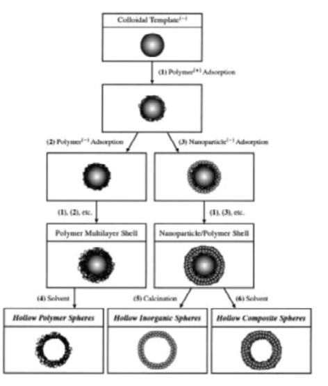
**Figure 6.** Schematic diagram for hollow capsule production by exploiting colloidal templating and self-assembly methods. Reprinted from Caruso, F. 2000, Chem. Eur. J., 6(3), 413-419, with permission from John Wiley and Sons.
