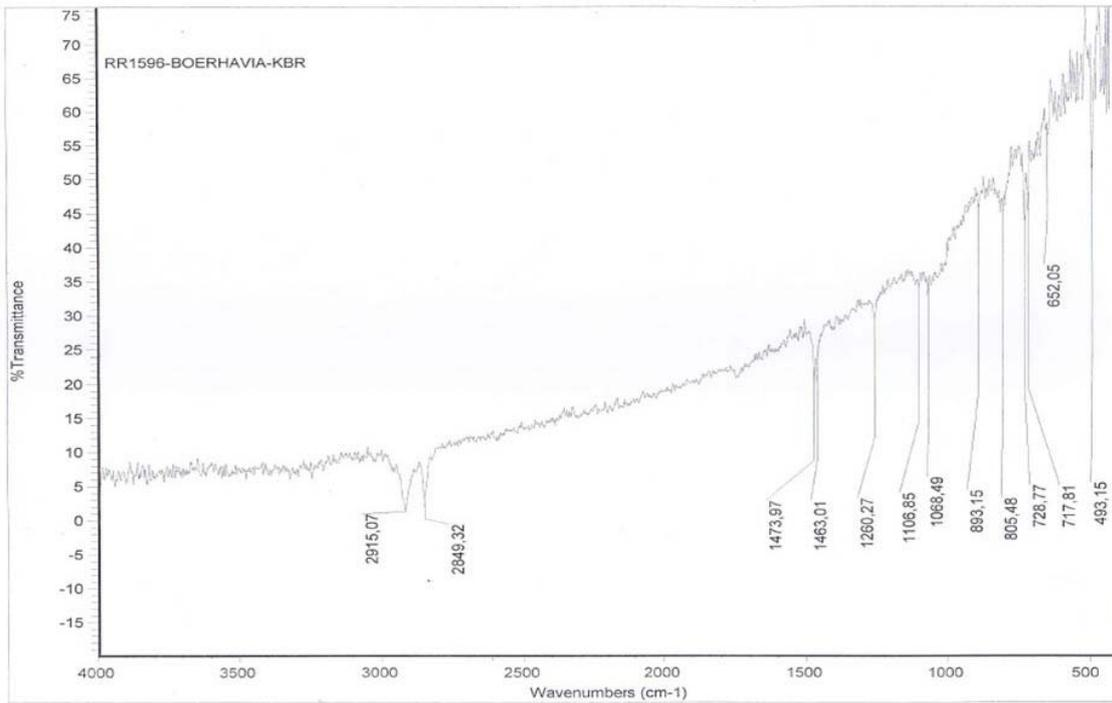
**Figure 2a.** FTIR analysis of chloroform fraction of hydro-alcoholic extract of root and stem parts of *Boerhavia erecta* L.
