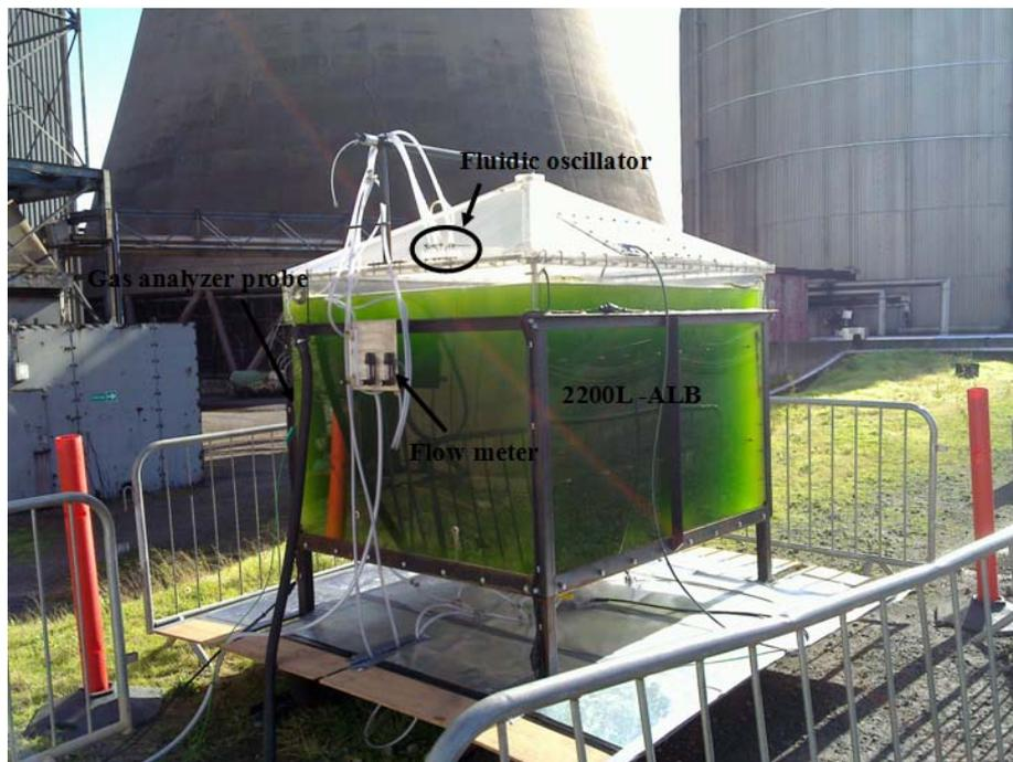
**Figure 1.** The setup of ALB for pilot trials.
