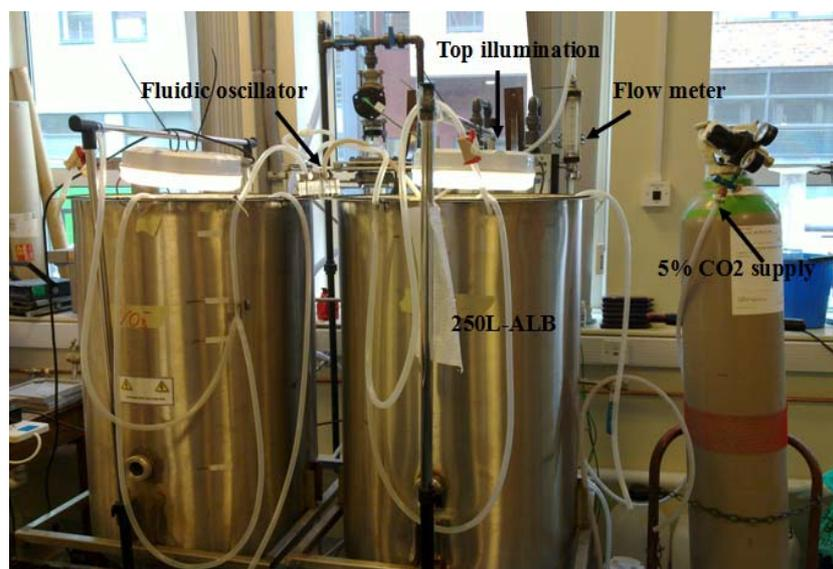
**Figure 7.** The laboratory setup of the 250 litre ALB culture.
