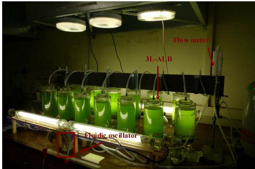
**Figure 3.** The laboratory setup of 13 ALB bench cultures of *Dunaliella salina*.
